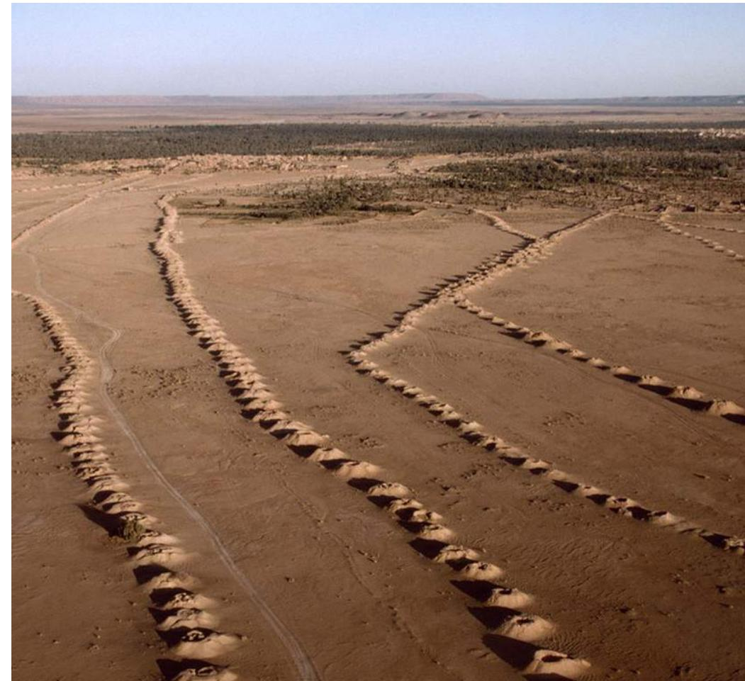
The Qanat system includes underground tunnels that collect water from surrounding mountains and transfer it to the plains and foothills where human settlements and production systems are located.
